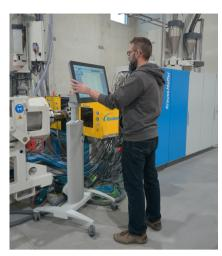
In addition to changing the pipe dimensions at the push of a button, QuickSwitch also handles the fine adjustment of pipe wall thickness and pipe centering. © KraussMaffei
