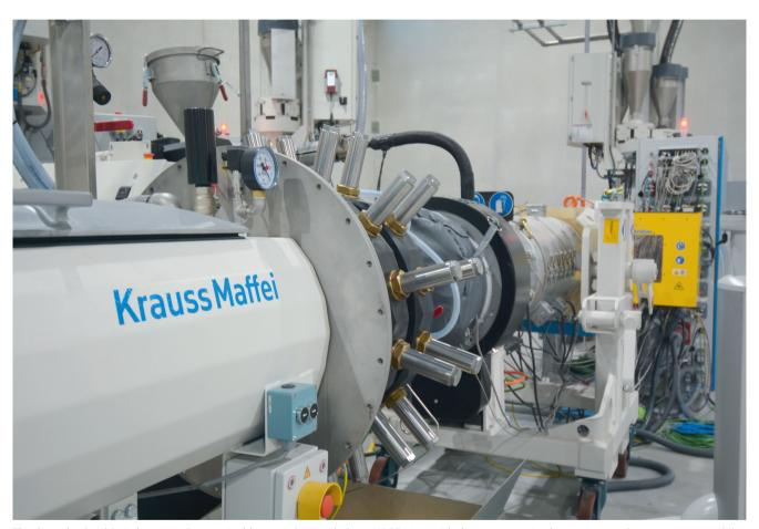
Thanks to the QuickSwitch system, Encoma is able to produce multi-layer HDPE pipes with diameters ranging between 25 and 63 mm on one and the same line. © KraussMaffei
