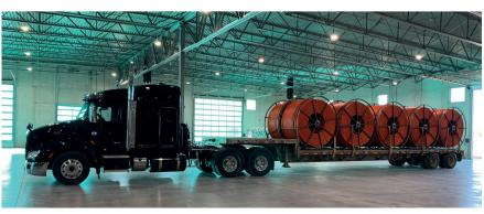
One of the first loads of three-layer HDPE pipes with a silicone inner layer produced by the industry newcomer Encoma in Canada. © KraussMaffei
